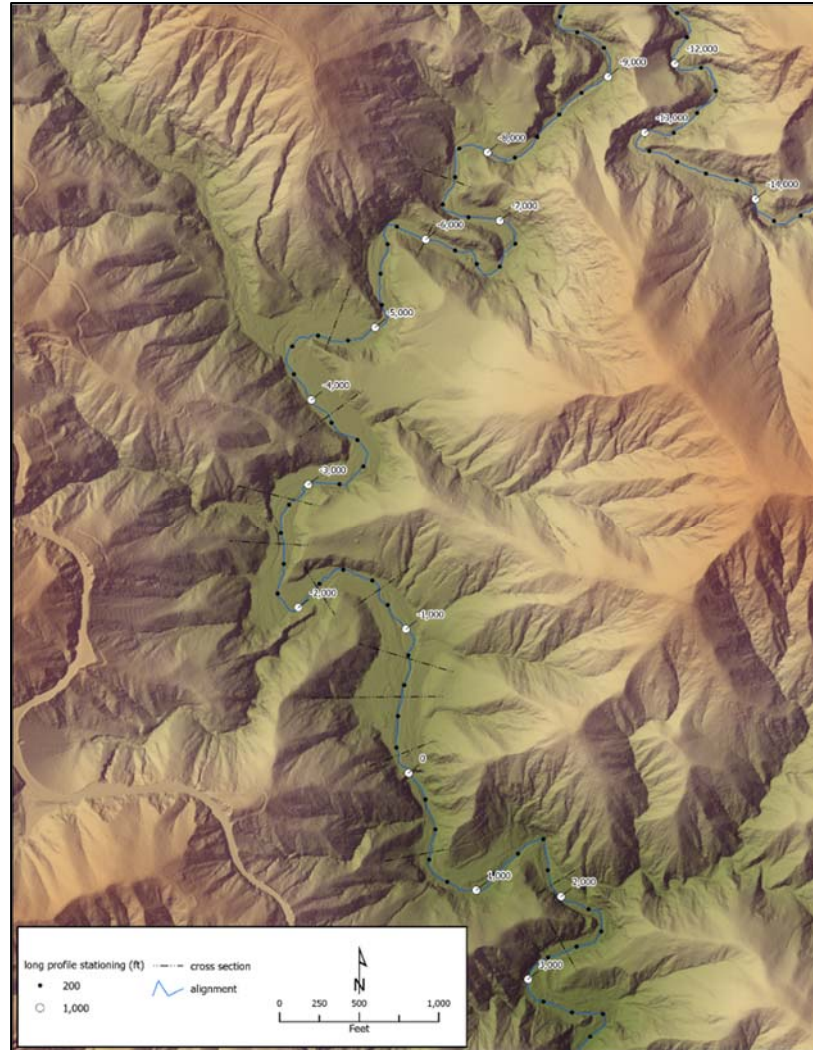
Figure 3-17. Shaded topography from the 2015-2016 LiDAR. Station numbering marks distance in feet upstream (negative) and downstream (positive) of the dam. Dashed black lines mark cross-sectional locations for volume calculations.
