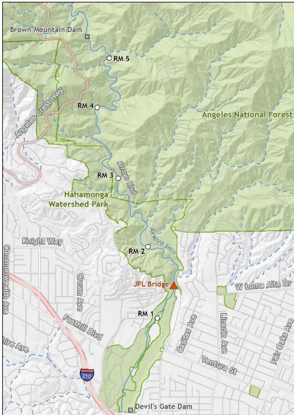
Figure 1-1 (cont.) b. The reach of primary concern for this report, from Devil's Gate Dam to Brown Mountain Dam. The reservoir deposits behind Brown Mountain Dam are present upstream to about river mile 6.7.
